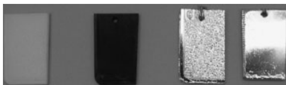
Figure 4. Direct metallization of plastics with PPy paints. From left to right: (a) raw ABS specimen, (b) PPy painted ABS specimen, (c) Cu-metallized PPy painted ABS specimen with rough surface and (d) Cu-metallized PPy painted ABS specimen with smooth surface.
